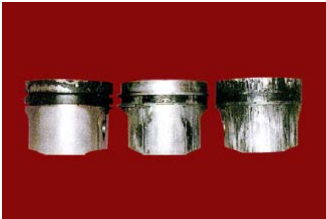
Fig. 56: Piston damage on this direct-injection engine resulted from improper cylinder jacket cooling. As shown by the middle piston, seizure usually begins in the skirt area while the top land escapes damage. The piston on the right shows further progression after skirt seizure.
