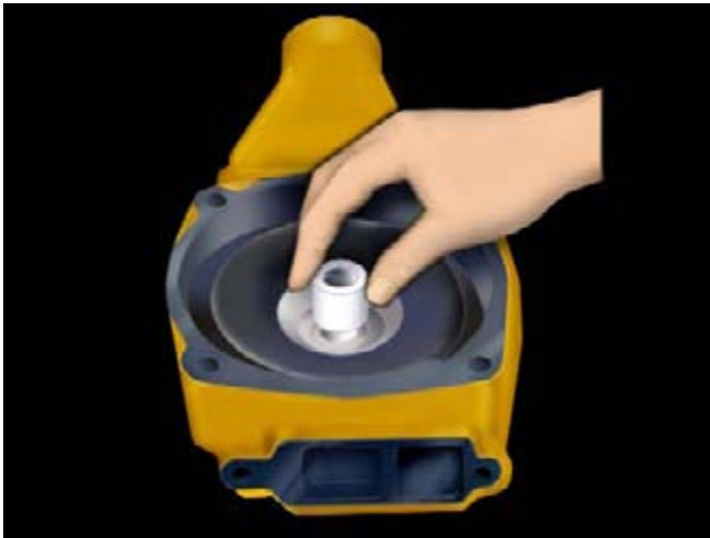
Fig. 77: Use a special tool to install the seal assembly.
