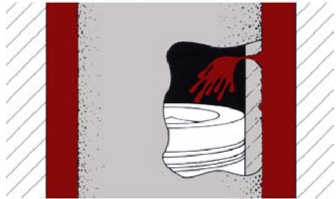
Fig. 47: Eventually, a pit can penetrate the cylinder wall and allow coolant to leak into the cylinder.
