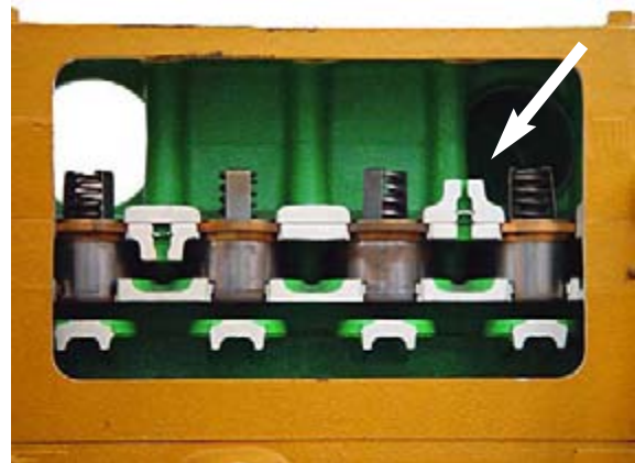
Fig. 68: Bleed hole in water temperature regulator housing.
