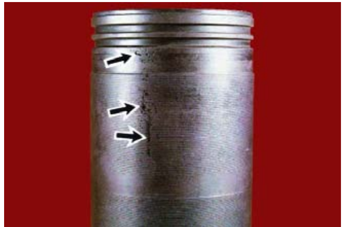
Fig. 44: Example of cylinder wall cavitation-erosion.
