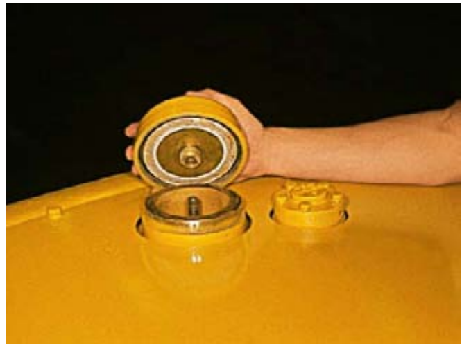
Fig. 63: Type of radiator cap held by studs.
