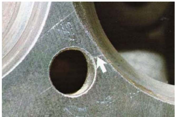
Fig. 55: Further inspection of the crack shows extension into the valve seat area.
