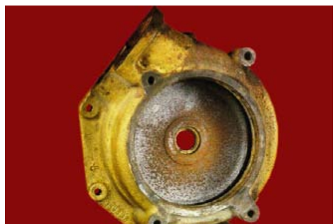
Fig. 51: Rusting inside water pump.
