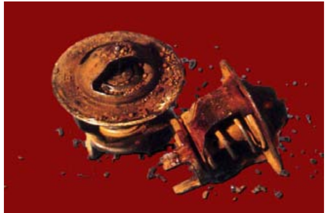
Fig. 42: Rust and scale deposits, due to the absence of supplemental coolant additive, caused temperature regulators to fail.
