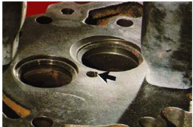
Fig. 54: Coolant-related overheating caused this crack in the cylinder head at the nozzle hole.
