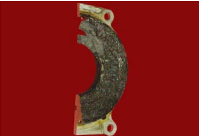
Fig. 49: Corrosion/erosion of aluminum Water Pump Adapter .
