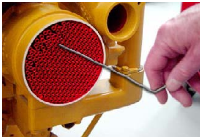
Fig. 74: Cleaning the tube bundles.
