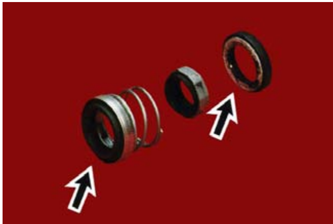
Fig. 38: Water Pump Seal Deterioration.
