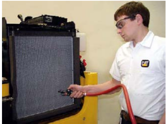
Fig. 69: Cleaning the radiator core (equipped with blower fan).
