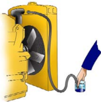
Fig. 65: Bottle test used to check for air or combustion gases in the cooling system.
