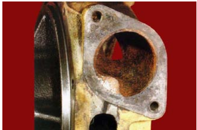
Fig. 43: Corrosion on a water pump passage due to lack of supplemental coolant additive in the cooling system.
