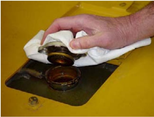
Fig. 13: Care must be taken during removal of the radiator cap.
