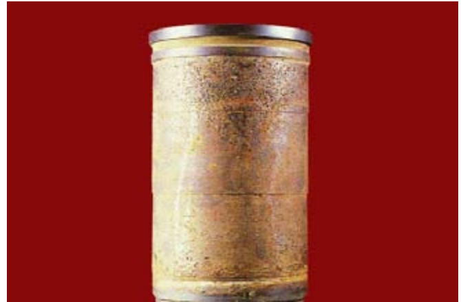
Fig. 50: Rust deposits on outside of cylinder wall surface.
