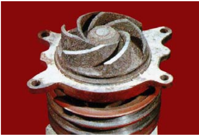
Fig. 53: Rust deposits on water pump impeller caused by lack of supplemental coolant additive.
