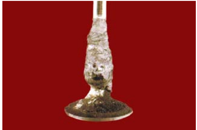
Fig. 57: Excessive carbon buildup on an intake valve. Carbon buildup can be caused by engine operating at cold temperatures.
