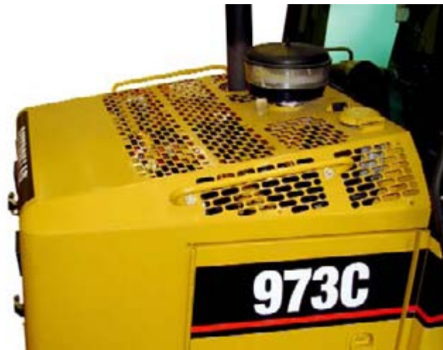
Fig. 108: Perforated Hood and Engine Side Enclosures.
